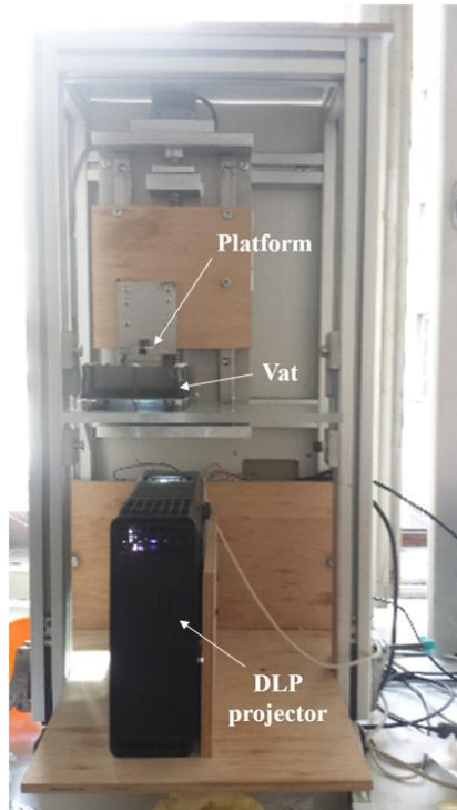
Figure 3: Custom built 3D DLP printer used in experiments.
