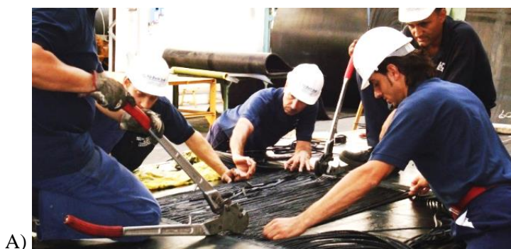
Figure 1-2: A) Preparation process of a steel cord splice [RI-Belt Sud S.R.L]; B) Layout of a 3-step steel cord splice
